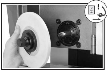
Figure 34. Wheel and hub removal.
